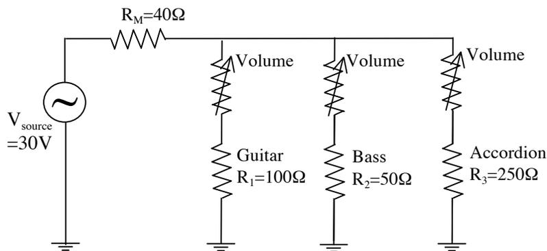
a) Say the guitar channel's volume knob is "all the way on", i.e. zero resistance, and the other two volume knobs are turned "off," i.e. "infinite" resistance. What is...
