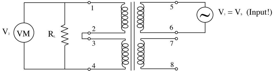
Fix the AC signal fixed at some voltage (or just leave it at 6V), press the "range" buttons on the signal generator to record the primary and secondary voltages for 10Hz, 100Hz, 1000Hz, and 10000Hz.
