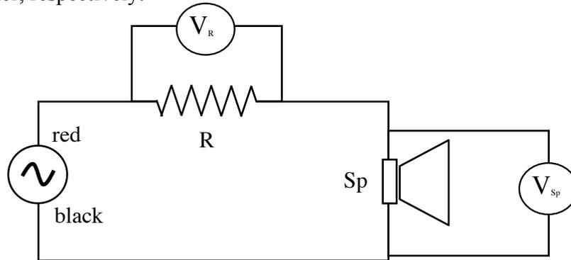
With this information, we can compute  $Z_{Sp}$  by noting that the relative lengths of the voltage vectors are *similar* to the relative lengths of the impedances (think of the impedance diagram and voltage diagram), i.e.  $R / V_R = Z_{Sp} / V_{Sp}$ .
