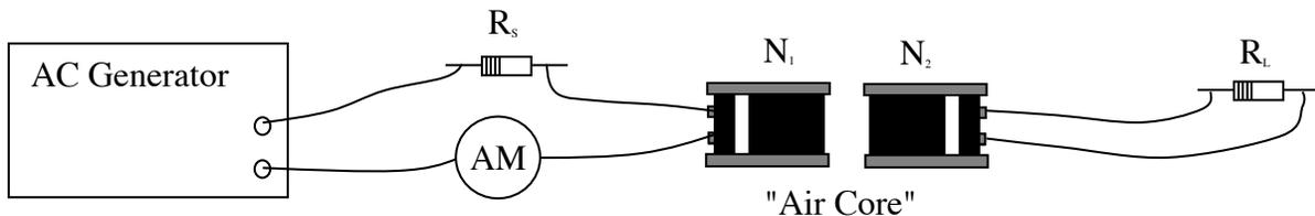
4. Make measurements for two different secondary coils, for the air core transformer shown above, as well as the following transformer configurations:
