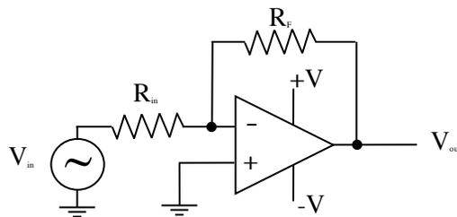
**Figure 1:** Closed-loop inverting amplifier diagram
