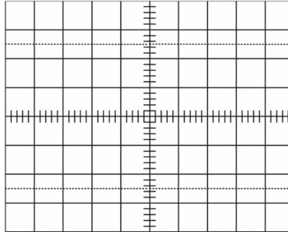
*Note that in this example, we have used the **maximum** Volts/div and Sec/div settings which still allow this (particular) complete waveform to be seen -- i.e. that make it "biggest" on the screen. Such settings allow us to make the **most accurate** readings of our signals, and should be used as a matter of **habit** when using the 'scope: **Always make the signal as "big" as possible, to get the most accurate readings.***
