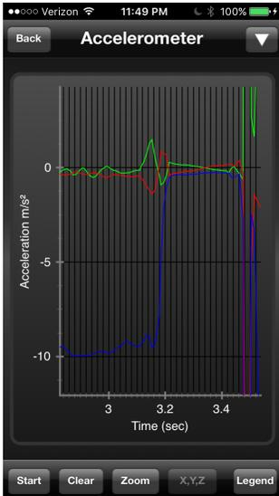
Step 7: Notice how there's a period during which the blue line drops to zero? That's the time during which the phone was in free-fall! You've just demonstrated the Equivalence Principle! Now, by reading the graph, find out how long the phone was in free fall. Call this time  $t$ , and write it in the following blank:
