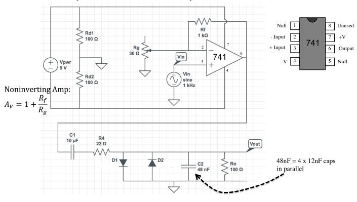
**Part 4. Rock!** Replace  $V_{in}$  with guitar input, run  $V_{out}$  into an amp, and rock out!
