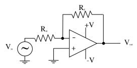
Figure 1: Closed-loop inverting amplifier diagram
