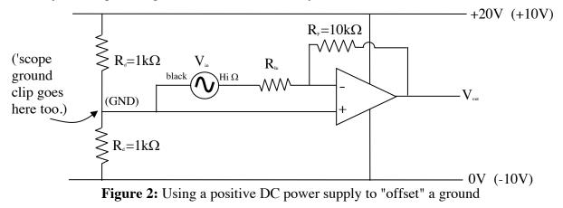
In the figure above, quantities in parentheses show the voltage values relative to the op amp. All signals will be measured relative to "(GND)", i.e. relative to the ground *for the op amp*, *not* the ground of the DC power supply.
