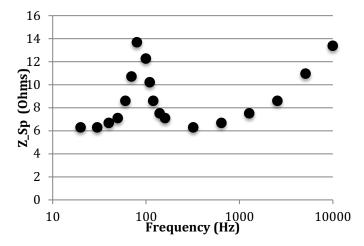
Quote: 'A speaker is not linear 8 ohms at all frequencies. We did this [test] at Prince's [studio]. The JBL 18" in the mains were rated at 600 watts 8 ohm, however the impedance dropped to 2 ohms at 60 Hz flowing A LOT more power at 60 Hz. No wonder the JBLs were so punchy because they flowed over 2000 watts at 60 Hz. This is also why Prince could literally blow the cone out of the basket. I had 18 spares to keep 8 in service.'
