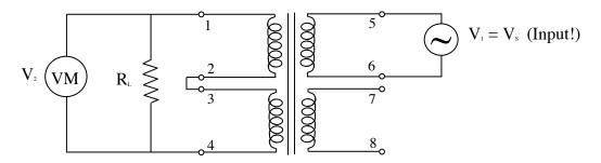
Fix the AC signal fixed at some voltage (or just leave it at 6V), press the "range" buttons on the signal generator to record the primary and secondary voltages for 10Hz, 100Hz, 100Hz, and 10000Hz.
