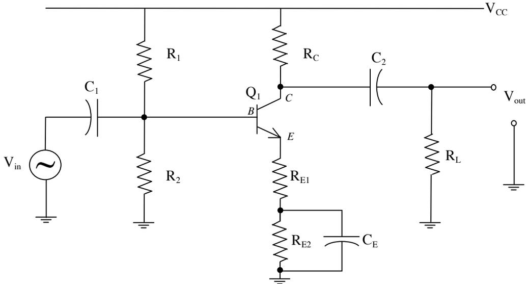
( $R_{E1}$  can either be an explicit resistor or it can represent the effective "resistance" which appears in real-world performance of diodes, i.e. the fact that there is a finite slope to the line on current-vs.-voltage graph for a diode, rather than an "instant" transition at 0.7V.)
