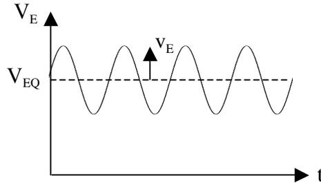
Note that because of the "diode drop" between the base and the emitter,  $V_E = V_B + 0.7V$ . The "AC part" of this equation tells us that  $v_E = v_B$ . A simple proof follows:
