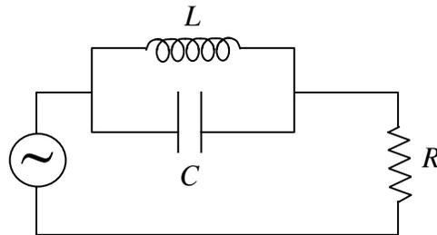
In the schematic shown,  $V_T = 100$  V,  $L = 1$  mH,  $C = 0.1$  mF, and  $R = 8 \Omega$ .
